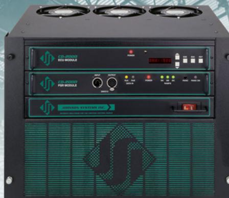
The CD-2000+ is a professional retrofit electronics package designed specifically for any vintage of Strand CD80 dimmer rack. This full-featured, state-of-the-art unit converts dual DMX inputs with protocol manager to 96 PWM and 128 DMX channels of output.
