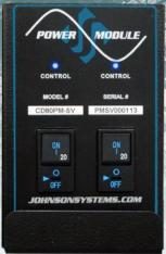
CD80 Non-Dim Power Modules allow existing CD80 and C21 dimmer rack owners to convert existing dimmer circuits to switched power circuits on the fly. These "plug & play" modules are a fast direct conversion for users requiring DMX non-dim control of devices/loads requiring pure sinusoidal AC power. Interchangeable constant and filler modules allow for increased flexibility and versatility.
