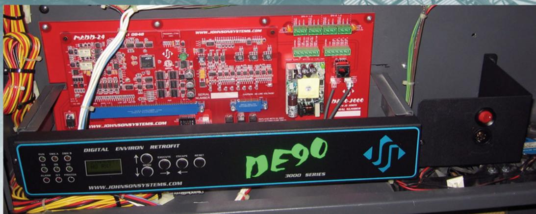
The DE90-3000 is a next generation retrofit electronics package designed specifically for Strand DE90 Architectural dimmer racks. The DE90-3000 will save significant \$\$\$ by replacing the aging control electronics of the existing DE90 dimmer rack making system replacement completely unnecessary. This full-featured, state-of-the-art unit provides a digital interface to modern lighting communication protocols.
